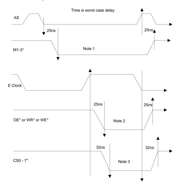
Note 1: M1-3 chip select delay is determined by 16V8 PLD rating and maybe 15ns. Note 2: OE, WR, and WE delay is determined by 16V8 PLD rating and maybe 15ns.
