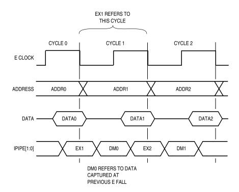
Figure 8-2. Queue Status Signal Timing (M68HC12)
