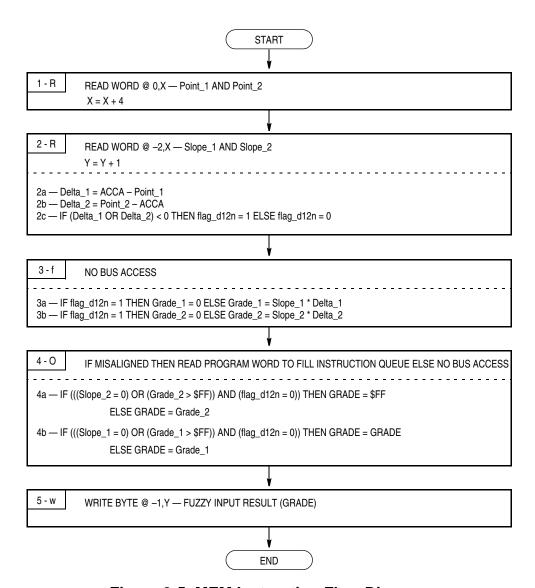
Figure 9-5. MEM Instruction Flow Diagram
