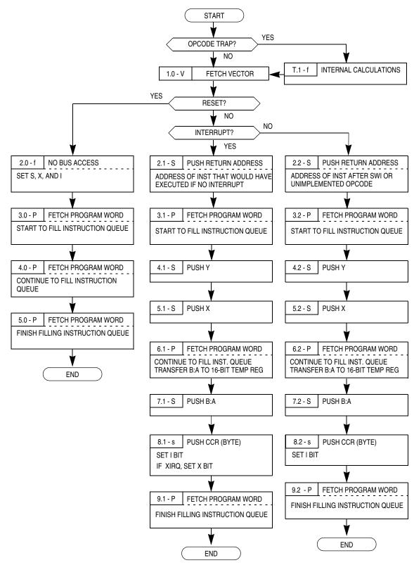
Figure 7-1. Exception Processing Flow Diagram
