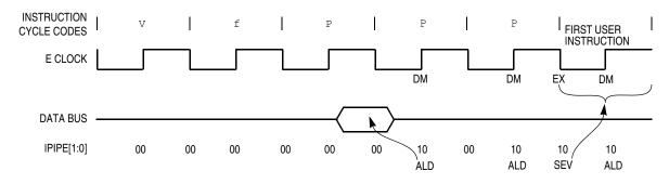
Figure 8-4. Reset Sequence for M68HC12
