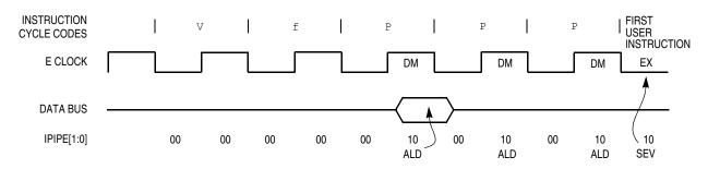
Figure 8-3. Reset Sequence for HCS12
