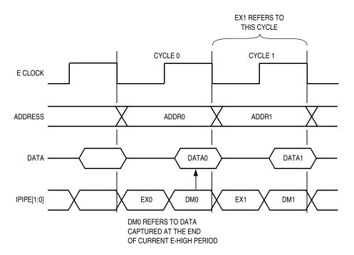
Figure 8-1. Queue Status Signal Timing (HCS12)
