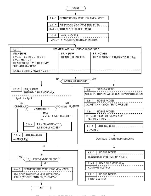
Figure 9-10. REVW Instruction Flow Diagram
