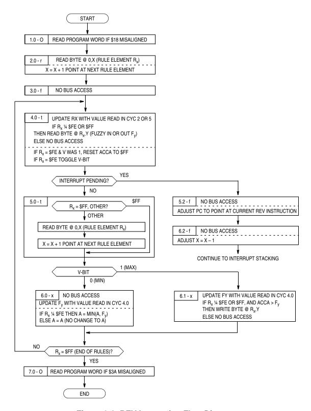
Figure 9-9. REV Instruction Flow Diagram
