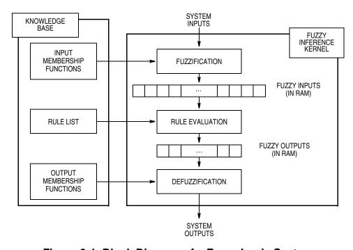
Figure 9-1. Block Diagram of a Fuzzy Logic System
