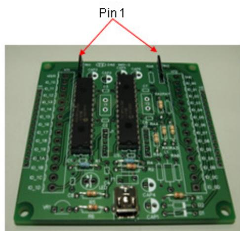
4. Assemble quartz crystal Y1,Y2(12MHz), C2, C3, C6,C7 (capacity 20pF).
