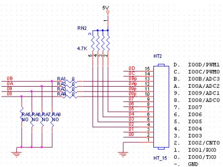
The pwm function makes it very simple to generate a programmable control voltage. It is also possible to use the pwm outputs without any filtering, the pwm output connected directly.
