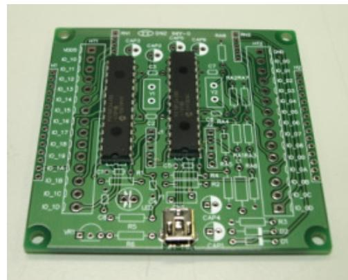
2. Assemble resistance R1,R4(the 10K ohm), RA1,RA2,RA3,RA4(the 0 ohms), R2(the 2K ohm), R3,R5,R6(the 300 ohm).
