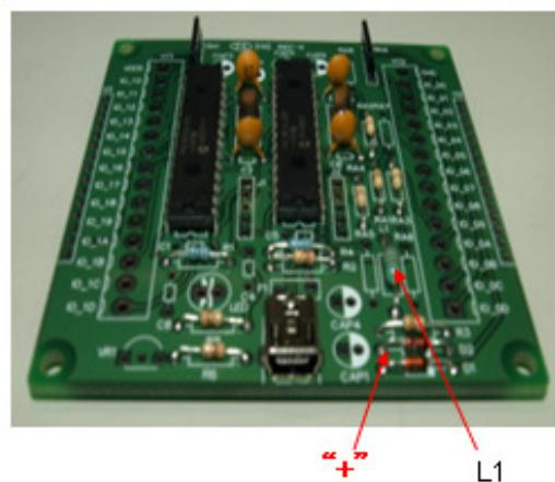
6. Assemble LED1 (LED, **attention polarity**). polymer resettable fuse FUSE1(0.5A) and VR1(TL431).
