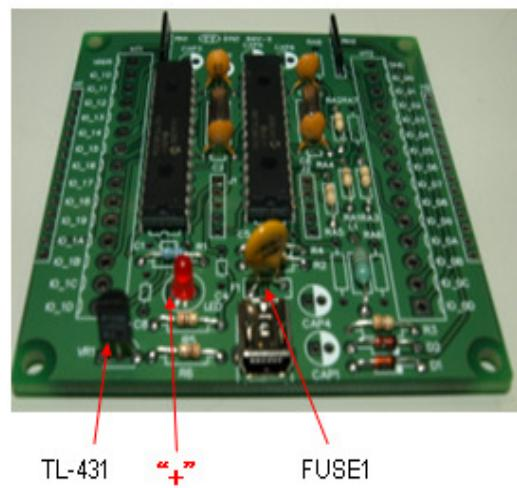
7. Assemble capacity CAP1, CAP4 (100uF, **attention polarity**), CAP2, CAP3, CAP5, CAP6 (10uF, **attention polarity**), C1, C5, C8(0.1uF), and Terminal Block Connector.
