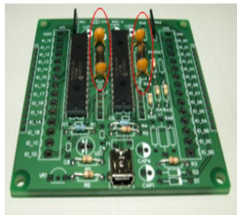
5. Assemble D1 and D2(the 1N4148 diode, **attention polarity**) and inductance L1(220uH).
