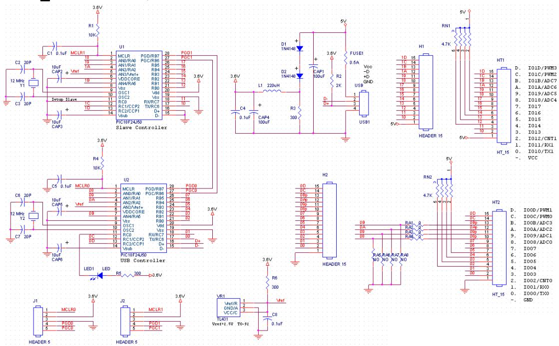
The 8 analog input channels (ADC0~ADC7) reference voltage is 2.5V. The analog input of ADC0 ~ ADC3 are resistor dividers. It means that you can control the ratio of resistor, manually. For example, RA1/RA8=10k/10k and the analog input voltage equals 2.5V, the ADC3 reads 0512. The analog input voltage equals 5V, the ADC3 reads 1023.(For a 10-bit ADC, the range is 0000 – 1023).
