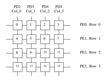
The pinouts of J6 for Wytec 4X4 membrane keypad are as follows:
