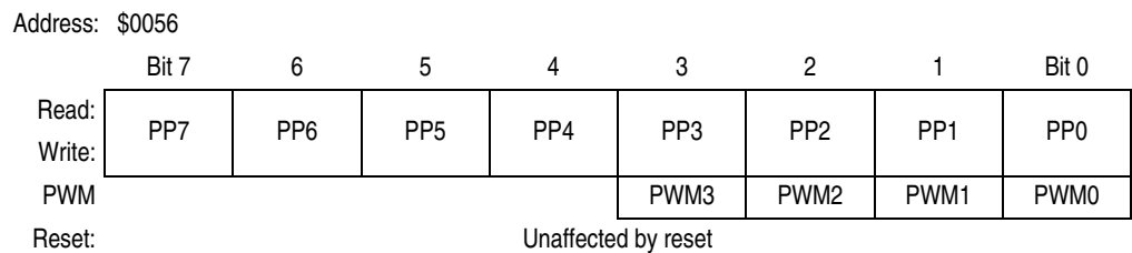
Figure 11-26. Port P Data Register (PORTP)
