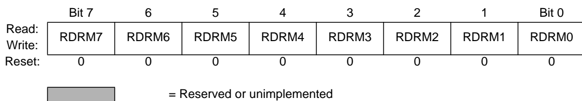
Figure 3-17 Port M Reduced Drive Register (RDRM)
